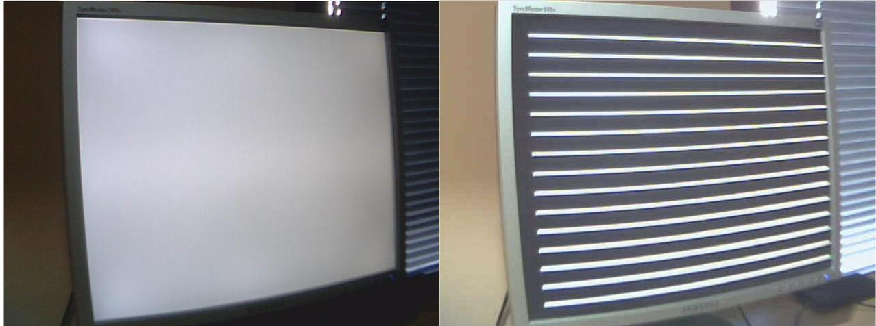
Figure 3.1. Image taken while LCD was filled with white color. Figure 3.2. Image taken while LCD was filled with lines.
